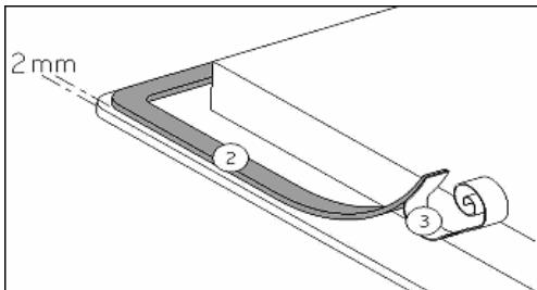
Stick the gasket (2) two millimetres from the external edge of the glass, after removing the protection sheet (3).
